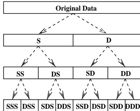
Figure 1: The wavelet packet decomposition for a 1-d signal decomposed to 3 levels. **S** and **D** refer to smooth and detail subbands.
