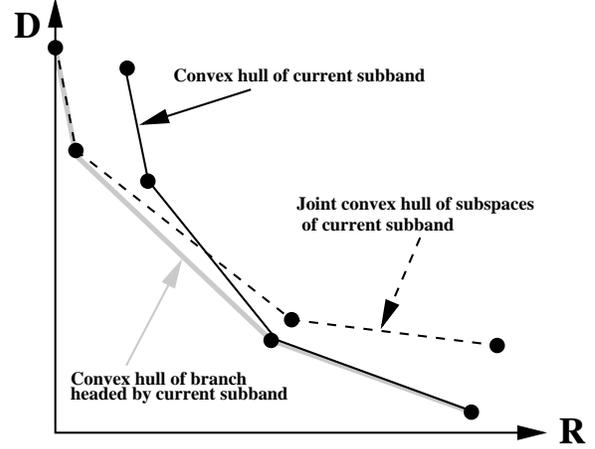
Figure 3: Optimal bit allocation/best-basis selection
