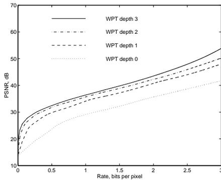
Figure 4: WPT/PTSVQ bit allocation as a function of WPT depth. The vector dimension is 4 for all PTSVQ's.
