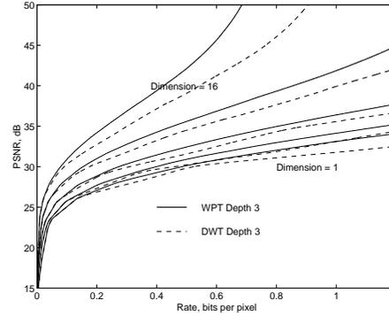
Figure 6: WPT/PTSVQ versus DWT/PTSVQ bit allocation for 3 levels of decomposition.
