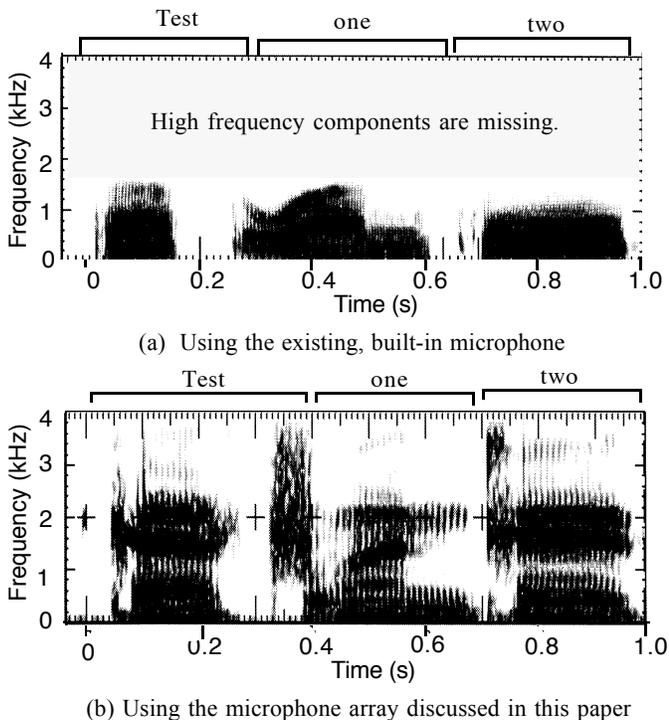
Fig. 6 - Speech spectra from the oxygen face mask. Note the presence of upper frequency components in Fig. 6(b) that are lacking in the muffled speech shown in Fig. 6(a). Both speech samples were spoken by the same person.
