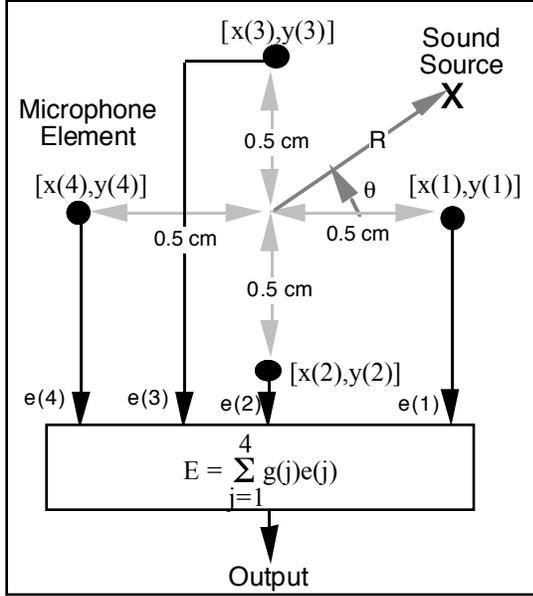
Fig. 1 — Generalized four-element microphone array configuration. A collinear array (shown in Fig. 3) is a special case of the array shown in this figure.
