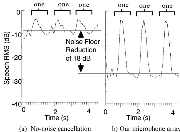
Fig. 5 - Histogram of speech RMS in the presence of E2C aircraft noise. As noted, our noise-canceling microphone improves the speech-noise ratio by 18 dB.
