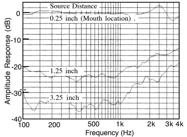
Fig. 4 — Measured frequency response from the prototype. The amplitude response approximates fairly well the theoretical response shown in Fig. 2. The near-field response is flat for frequencies below 2 kHz, and far-field response has a high-pass characteristic as in the theoretical response. The attenuation at one inch from the mouth location is as much as 24 dB which can be further raised by using a more refined summing amplifier and even better matched microphone cartridges.
