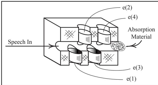
Fig. 3 - Cross-sectional view of the microphone array housing used in our prototype where four microphone elements are spaced collinearly at 0.5 cm apart.
