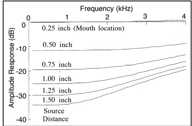
Fig. 2 — Theoretical frequency response of the microphone array in which four microphone elements are placed collinearly 0.5 cm apart. Eq. (5) is used to plot these curves.
