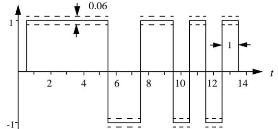
Figure 3. 13-bit Barker-coded signal with input mask
