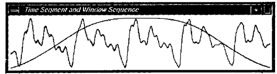
Figure 2: Segment of input audio data overlapped with the analysis window and the reconstructed sub-segment (first half) of decoded audio.
