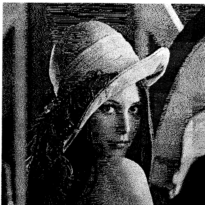
Figure 2: Halftone generated using Floyd-Steinberg error diffusion. The compression ratio achieved using a JBIG coder is 1.89. The printing resolution is 150 dpi.
