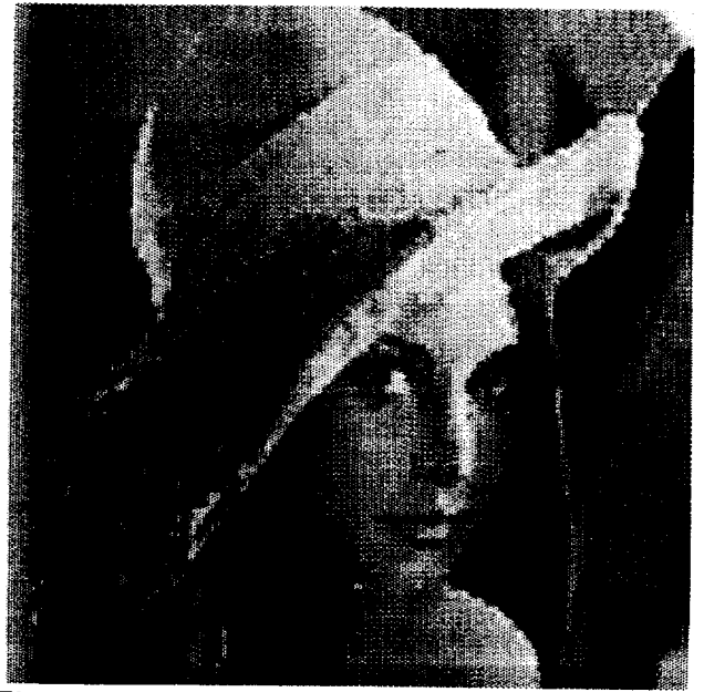
Figure 3: 0.1 bit/pixel without entropy coding, 5 subbands. PSNR is 27.53 dB
