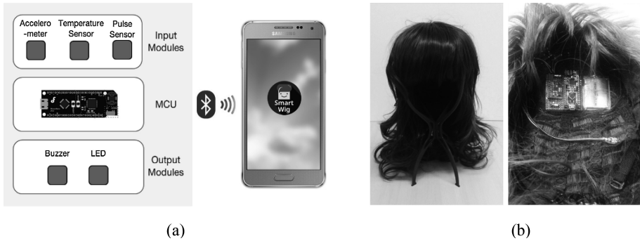
Fig. 1. (a) Our system consists of three parts (Input module, MCU, and Output module, which communicates with a smartphone application via Bluetooth). (b) Prototype using a wig.
