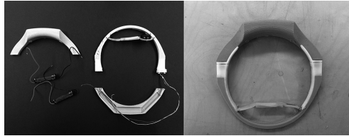
Fig. 8. The picture on the left shows a dissembled view of the fabricated model. The picture on the right shows an assembled one.
