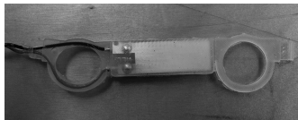
Fig. 9. The picture shows a finished silicone part with flex sensor in it. The two holes on both sides are for microphones.
