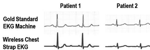
Fig. 3. Comparison of simultaneously recorded EKG traces from the standard wired EKG machine and the wireless chest strap (i.e. the Bioharness) of the WMMS.
