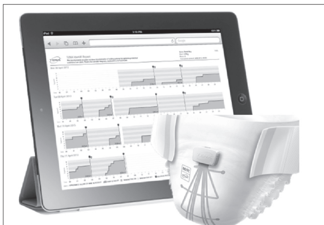
Fig. 2. Illustration showing the idea of the innovation tested: a disposable protective product with sensors and logger along with an example of graphic report of data. Picture courtesy of © Copyright 2015 Svenska Cellulosa Aktiebolaget SCA.
