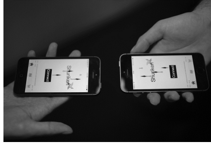
Fig. 1. An example showing the mechanism to point the devices together with the “button” method to confirm the device link.
