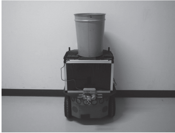
Fig. 5. Developed trash-box type robot
