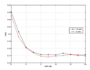
**Fig. 2.** MSE for a scenario with 8 transmit antennas and 2 receive antennas.
