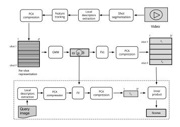
**Fig. 1**. Complete pipeline of our proposed architecture. Dotted line encloses the query stage described in Section 3.2.
