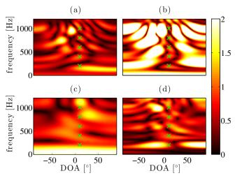
Fig. 1: Filter responses for (a) IAA based on noise covariance matrix estimate  $\widetilde{\mathbf{Q}}_{\omega_{t,s}}$  (b) IAA based on covariance matrix estimate,  $\widetilde{\mathbf{R}}$  (c) APES based estimate with  $N_t=20$ ,  $M_t=10$ ,  $N_s=10$ , and  $M_s=5$  (d) APES based estimate with  $N_t=224$ ,  $M_t=20$ ,  $N_s=10$ , and  $M_s=10$ . Harmonics of desired signal are marked by green crosses. The average input SNR is  $10~\mathrm{dB}$ .
