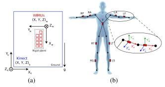
Fig. 1. Configuration of our testing platform. During the initialization step (a) the spatial coordinate system of each inertial sensor are the same and this spatial reference is aligned with the Kinect one. (b) Each WIMU is fixed on the subject's bones:  $X_w$  is fixed along the bone toward the smaller joint. The black skeleton is a representation of our fused skeleton.
