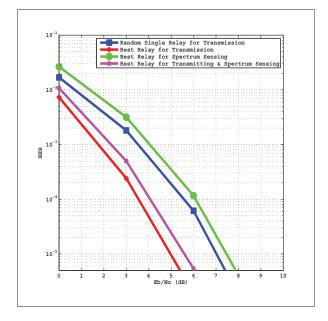
**Fig. 3.** Error performance curves for 4 different scenarios for Rician fading channel.
