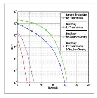
**Fig. 2**. Error performance curves for 4 different scenarios for Rayleigh fading channel.
