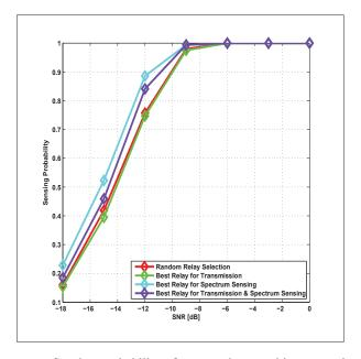
**Fig. 5**. Sensing probability of cooperative cognitive network for Rician fading channel.
