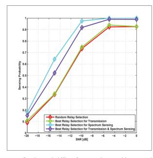
**Fig. 4**. Sensing probability of cooperative cognitive network for Rayleigh fading channel.
