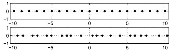
**Fig. 1.** Example of samples time-location in a) uniform sampling, b) nonuniform sampling - visible gaps and clustering of samples.
