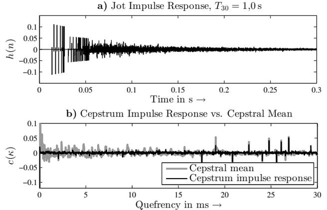
**Fig. 2.** a) Time signal of an impulse response generated using Jot’s reverberator [14]. b) Cepstral mean computed from an anechoic signal reverberated with the impulse response from a) and the actual cepstrum of the impulse response from a).
