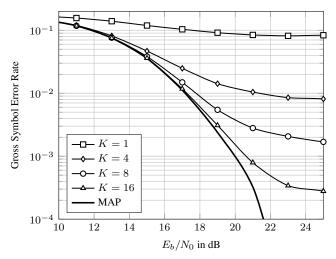
**Fig. 3.** Gross SER of zero-augmented BPSK and sparse K-Best detection for an underdetermined scenario.
