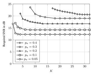
**Fig. 4.** Required SNR for target Gross SER of  $10^{-2}$  with varying K.
