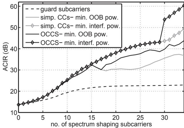
Fig. 3. Mean ACIR caused by the SU transmitter to the PU receiver vs. the number of spectrum shaping subcarriers.
