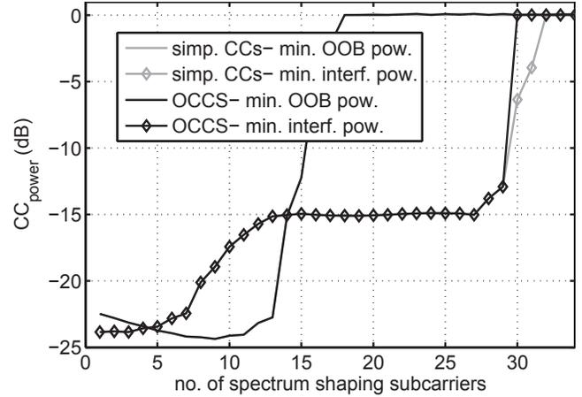
Fig. 4. Mean CC power normalised to the mean DCs power for the CC-based scenarios vs. the number of CCs.
