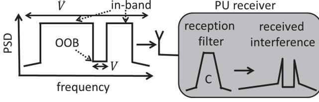
Fig. 1. The SU signal PSDs before and after the PU RX filter.
