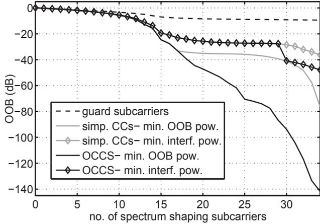
Fig. 2. Mean OOB power observed in the PU band vs. the number of spectrum shaping subcarriers.
