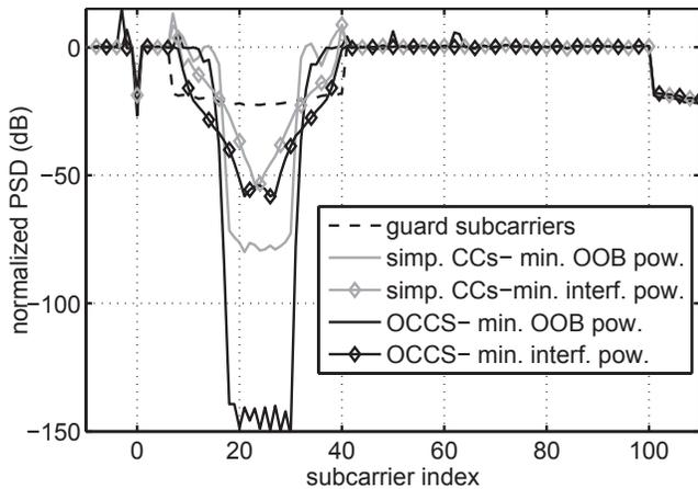
Fig. 5. Normalized PSDs for the considered scenarios at the PU RX antenna (before filtering);  $\beta = 34$ .
