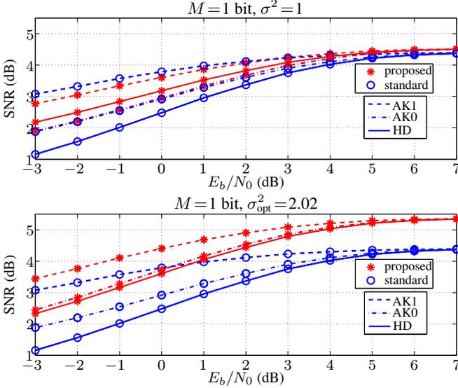
**Fig. 5:** Simulation results for  $M = 1$  bit quantized Gaussian AR(1) samples with correlation coefficient  $\rho = 0.9$ .
