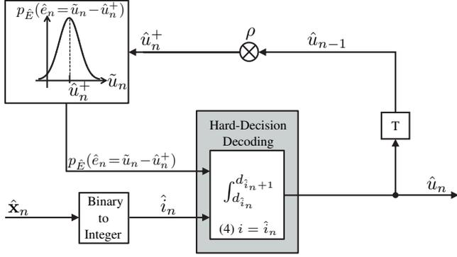
**Fig. 3:** Block diagram of the newly proposed receiver with hard-decision decoding (HD).
