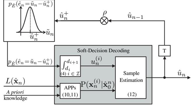
**Fig. 4:** Block diagram of the newly proposed receiver with soft-decision decoding (SD).
