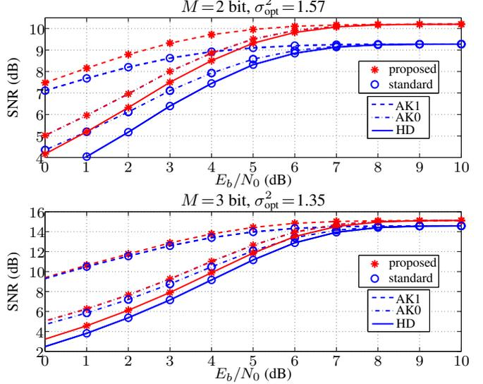
**Fig. 6:** Simulation results for  $M = 2$  bit,  $M = 3$  bit quantized Gaussian AR(1) samples with correlation coefficient  $\rho = 0.9$ .
