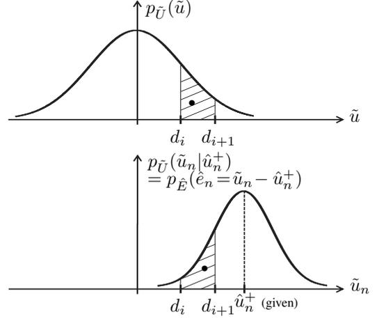
Fig. 2: Unquantized sample PDF and shifted PDF of the receiver-sided prediction error.
