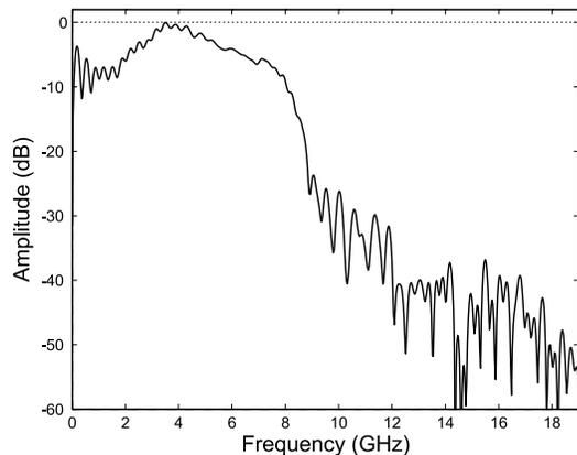
Fig. 4. Magnitude of the spectrum of the chirped impulse.
