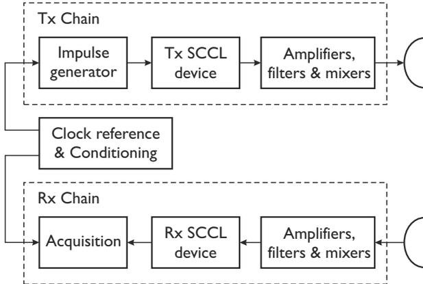
Fig. 1. Proposed architecture for a chirped IR-UWB radar.
