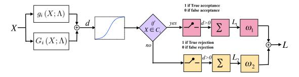
Figure 3.2: Minimum Verification Error architecture
