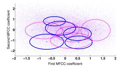
Figure 4.3: Scatter plot comparison between noisy and clean features: the continuous ellipses show the GMM component of a speaker model in clean conditions; the dotted ellipses represent the same recordings with added noise at 0 dB.
