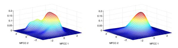
Figure 4.4: Example of model distribution for one speaker, a) speaker model in clean conditions b) speaker model in noisy conditions (0 dB SNR).
