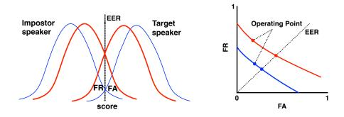
Figure 4.5: Score distributions and DET curves for two scenarios: a) blue line represents the clean condition, b) red line shows the noisy condition.
