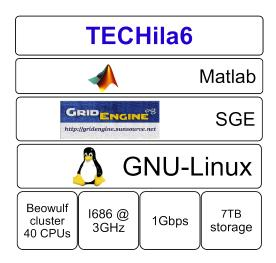
Figure 5.1: Infrastructure used by the Speaker Verification System
