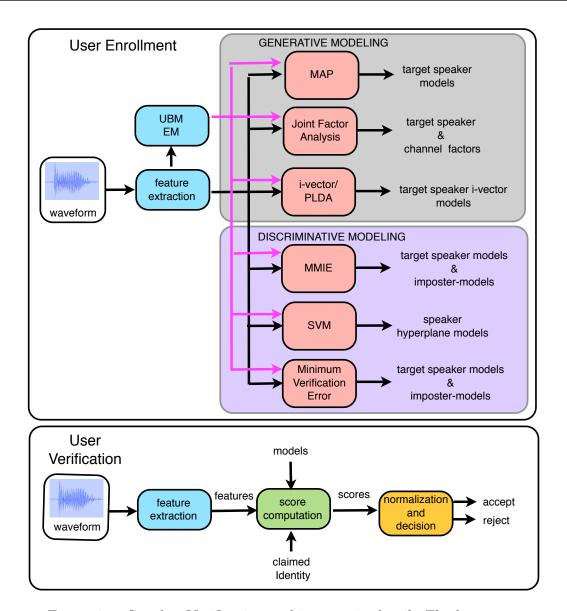
Figure 2.1: Speaker Verification architecture in detail, *The big picture*
