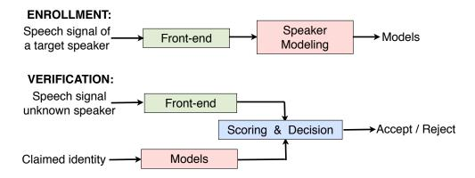
Figure 1.1: Simple Architecture of a Speaker Verification System
