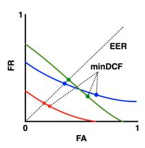
Figure 2.5: Detection Error Tradeoff curve
